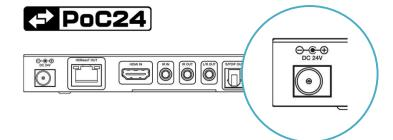
Ability to connect a single PSU to either transmitter or receiver adding extra convenience to your install. 24V PoC is standardardised accross all Netvio HDBaseT products.
